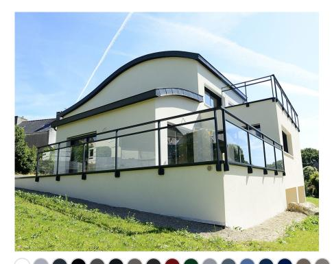
Be bold with transparency with the Mel guardrail! Its glazed base is ideal for letting light through. For those who are more reserved, you can opt for opaque or tinted glazing. Safety level: its multi-layered glazing, held together by a PVB film, keeps the glass pieces together in the event of glass breakage.
